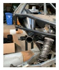
You will have to shorten the Front Right (ex side) body cage pin to make sure it doesn't hit the pipe. We have just left you enough room to get the pipe through and get a clip into the closest pin hole. The cut off all extra length beyond this pin hole.
