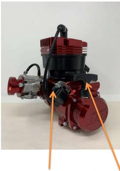
Coil with the two terminals for remote kill switch hook up. (zen style)
