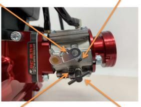
Low Speed mixture adjustment screw Base setting:- 1 3/8 turns out
