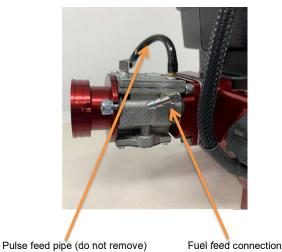
Note: This carburettor has only one connection to the fuel tank. This is the fuel feed tube which must have an in tank filter fitted.
