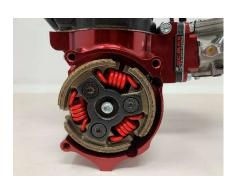
A New 78mm fibre clutch will measure around 75.9mm outside diameter. You can wear this down until the fibre pads are almost down to the metal before youll need to replace it.
