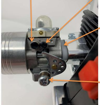
Idle Speed Adjustment Screw
