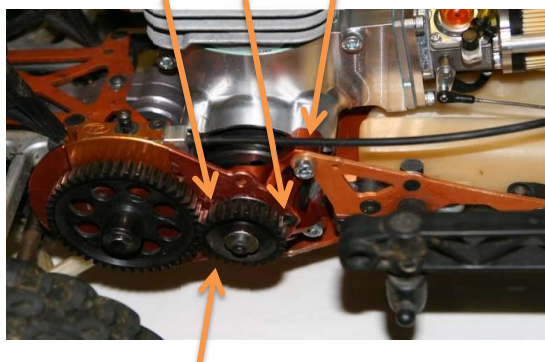
Right side mounting bolts (2 behind pinion)
