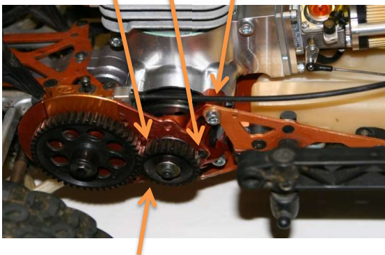
Right side mounting bolts (2 behind pinion)
